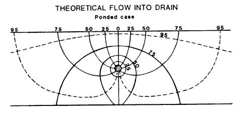
Figure 8. Theoretical flow into a drain.
