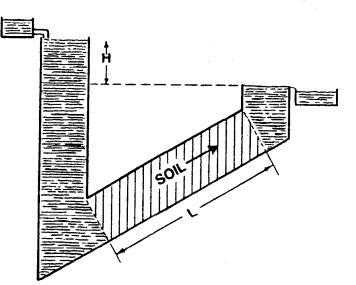
Figure 7. Water movement as a result of potential difference.
