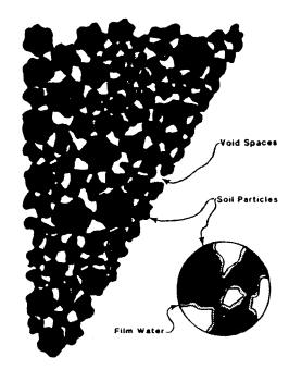
Figure 3. Characteristic structure of granular soil.
