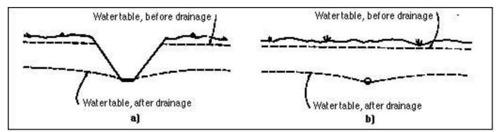
Figure 1. Water table level before and after drainage inprovement: a) surface drainage ditch; b)subsurface drainage pipe. (adapted from USDA-ERS, 1987)
