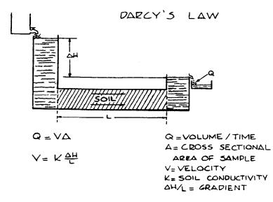
Figure 6. Experiment for hydraulic conductivity measurement.
