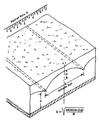
Figure 9. Steady-state drainage condition.
