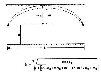
Figure 10. Falling water table drainage condition.
